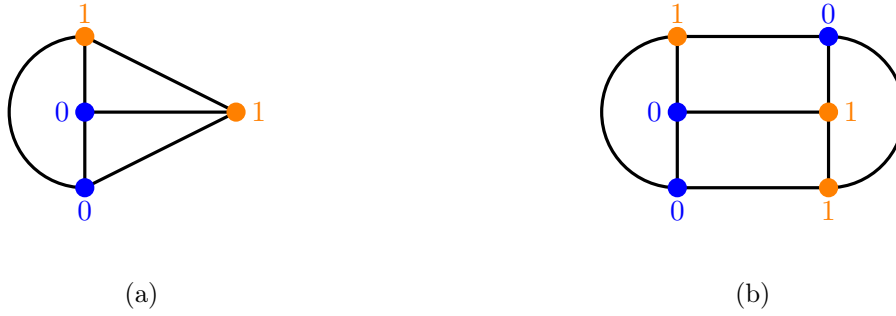
Figure 5.2: Obtaining the candidate solution for the original graph in Figure 5.1 after the two variable eliminations specified there were performed. (a) An optimal solution for the classical problem instance associated with H_G^{\text{Is}} = -Z_1Z_3 - 2Z_1Z_5 + Z_1Z_4 - Z_3Z_4 - Z_3Z_5 + Z_4Z_5 + 2I , i.e., the final Hamiltonian in Figure 5.1. This solution was obtained via brute-force calculation. (b) The final output of \text{RQAOA}_1^{\text{Is}} applied to the original graph in Figure 5.1. We assign 0 to the vertex 2 since it was negatively correlated with vertex 1 which had been assigned the value 1 in the solution in (a). After that, we assign 1 to the vertex 6 since it was negatively correlated with vertex 5 which had been assigned the value 0 in the solution in (a).
