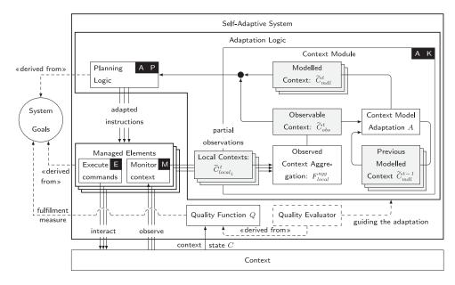
Fig. 4. The proposed logical architecture. The different components in the self-adaptive system are marked in order to signify where different phases of the MAPE-K loop are implemented. The grey boxes are not functional components; instead, they are the context models that can be seen as separate artefacts. We have kept them as separate components in the architecture, as they have a central role in the solution and clarify what information passes from one component to another.
