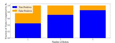
Fig. 6. The TP fraction of the tasks completed by robot 1 for a FP probability of 50%. The one robot case does not use KA whereas the combination aggregation scheme is used for two and five robot case. The results have been averaged over the five seeded runs.
