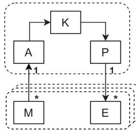
Fig. 2. Master-Slave pattern of the MAPE-K loop.
