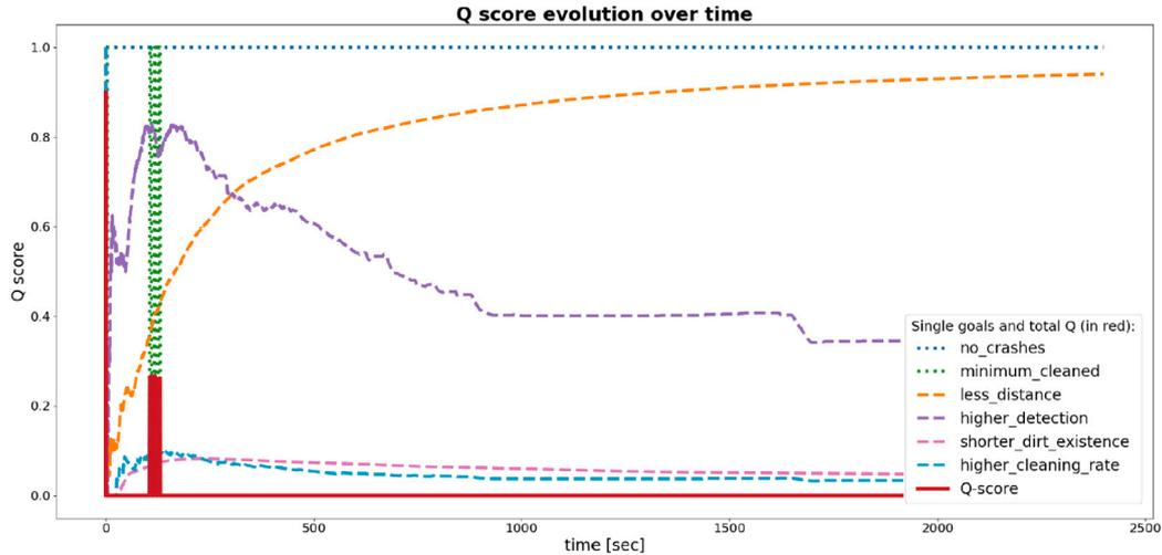
(a)  $Q$  score for too high spawning rate (achieve 10% cleaning rate is not possible).
