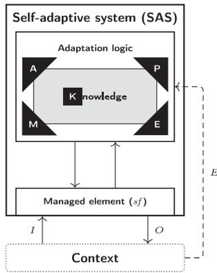
Fig. 1. Updated conceptual model of a self-adaptive system from [3].
