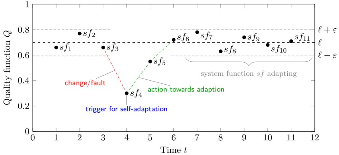
**Figure A.2:** The process of self-adaptation, modified from [96].
