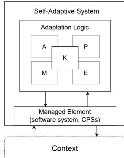
**Figure 1.1:** Conceptual model of a self-adaptive system [118, 66].
