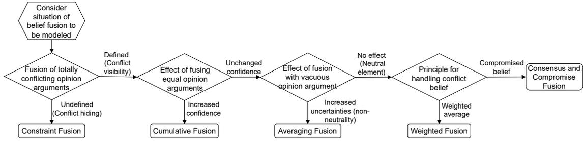
**Figure 2.7:** Decision process for selecting the most adequate fusion operator, adopted from [61].
