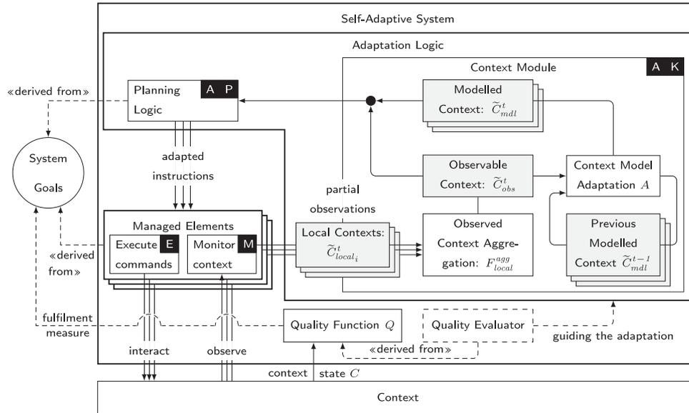
Fig. 4. The proposed logical architecture. The different components in the self-adaptive system are marked in order to signify where different phases of the MAPE-K loop are implemented. The grey boxes are not functional components; instead, they are the context models that can be seen as separate artefacts. We have kept them as separate components in the architecture, as they have a central role in the solution and clarify what information passes from one component to another.
