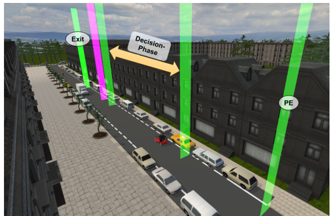
Fig. 2: Trigger points for the AV within an investigation scenario: Pre-information (PE), Decision phase, virtual stop line and the exit scenario trigger
