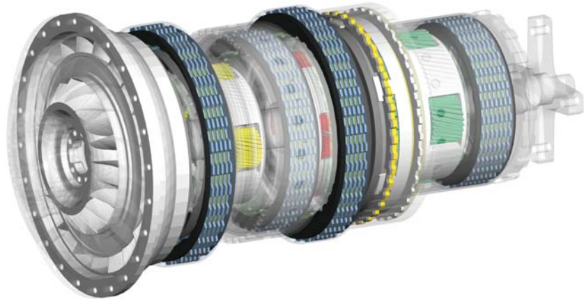
Figure 6.1: Model rendering of the automatic transmission, CCDC substituting brake C (B06)
