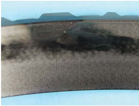
(a) Photograph of a hotspot on the friction surface of the steel cone
