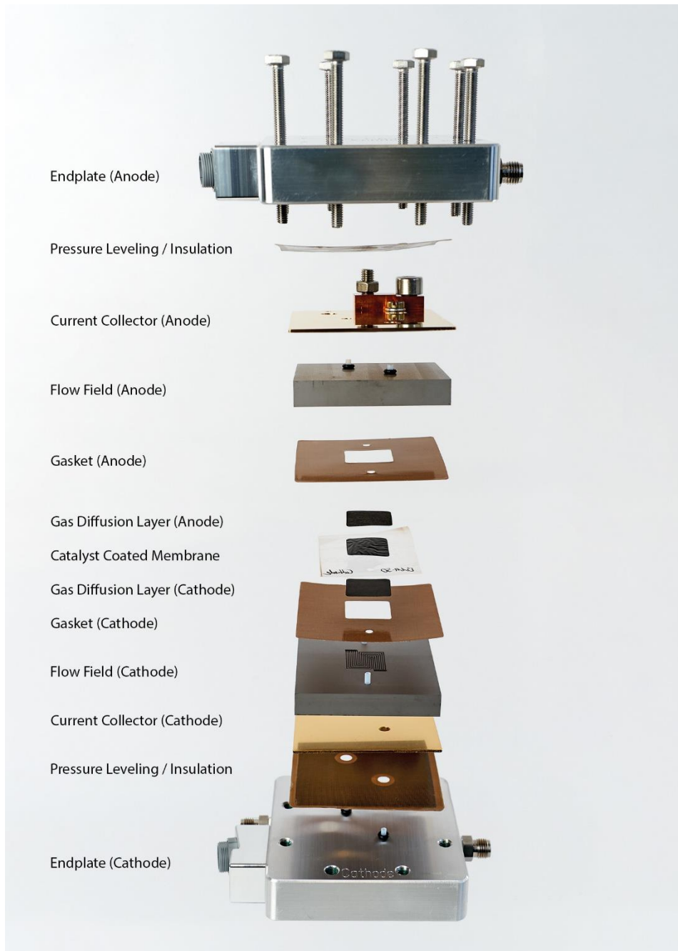
Figure 1.1: Schematic illustration of the main components of a 5 cm 2 single cell PEMFC. Curtesy of Dr. Björn M. Stühmeier.
