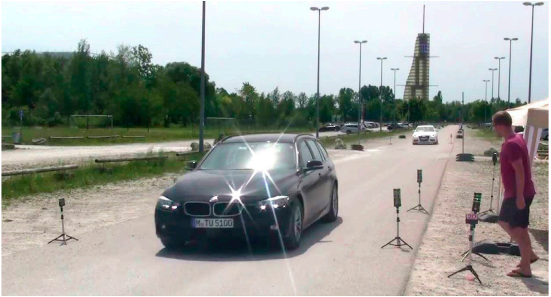
Figure 2. Participant initiating crossing in the test track environment. Light barriers served to register the movement of stepping forward and to measure the speed and distance of the vehicles.
