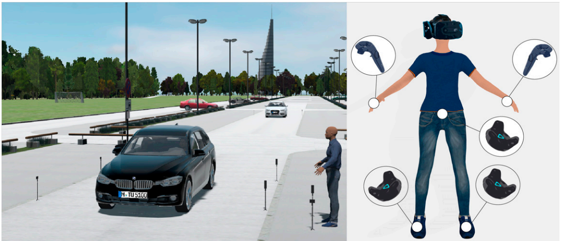
Figure 3. Virtual environment modeled after the test track (left) and the positions of tracking equipment used to visualize the ego avatar in the HMD condition (right). In the CAVE condition, virtual representations of the SMARTSPEED timing gates in front of the participant were replaced by physical substitutes, since the lack of a floor projection rendered them invisible in VR. CAVE = CAVE automatic virtual environment; HMD = head-mounted display; VR = virtual reality.
