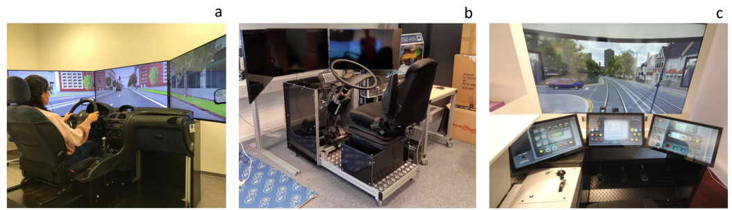
Figure 1. Driving simulators for the different modes: (a)—Passenger cars, (b)—Trucks (heavy vehicle simulator), (c)—Trams.
