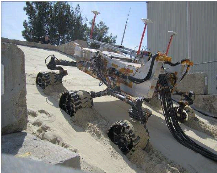
Figure 2.1: Mars Science Laboratory (MSL) engineering model tested on dry, loose sand [Con+12].
