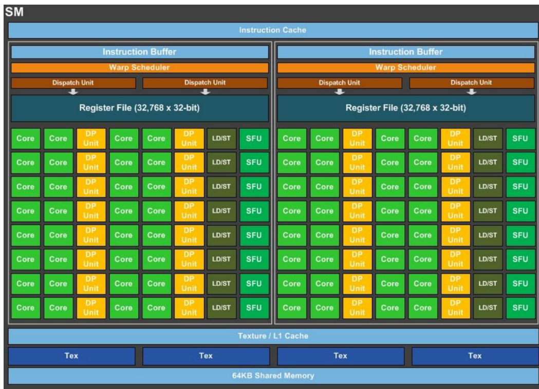
Figure A.1.: SM-architecture for Pascal [67]
