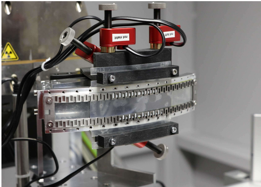
Figure 4.9: Photo of a manipulator-tape-based mount which is used to simultaneously bend and adjust a grating mounted on a manipulator-tape. The tape allows motorized stages to push and pull the grating to the correct position. After adjustment is finished the mechanical parts can be removed and the protruding flaps of the manipulator tape can be cut away. Then the aluminum mount and the bent grating are an extremely compact and stable construction.
