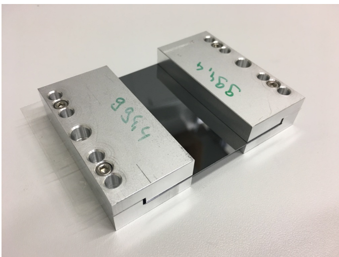
Figure 4.5: Photo of a 1 mm thick silicon wafer bent to a radius of 995 mm. The substrate has been cut to a rectangular shape and is approximately 65 mm wide. In [96], recently silicon-based absorption gratings produced by a new fabrication process have been demonstrated. There a centrifugal tungsten deposition has successfully been used to fill the gratings with the absorber material.
