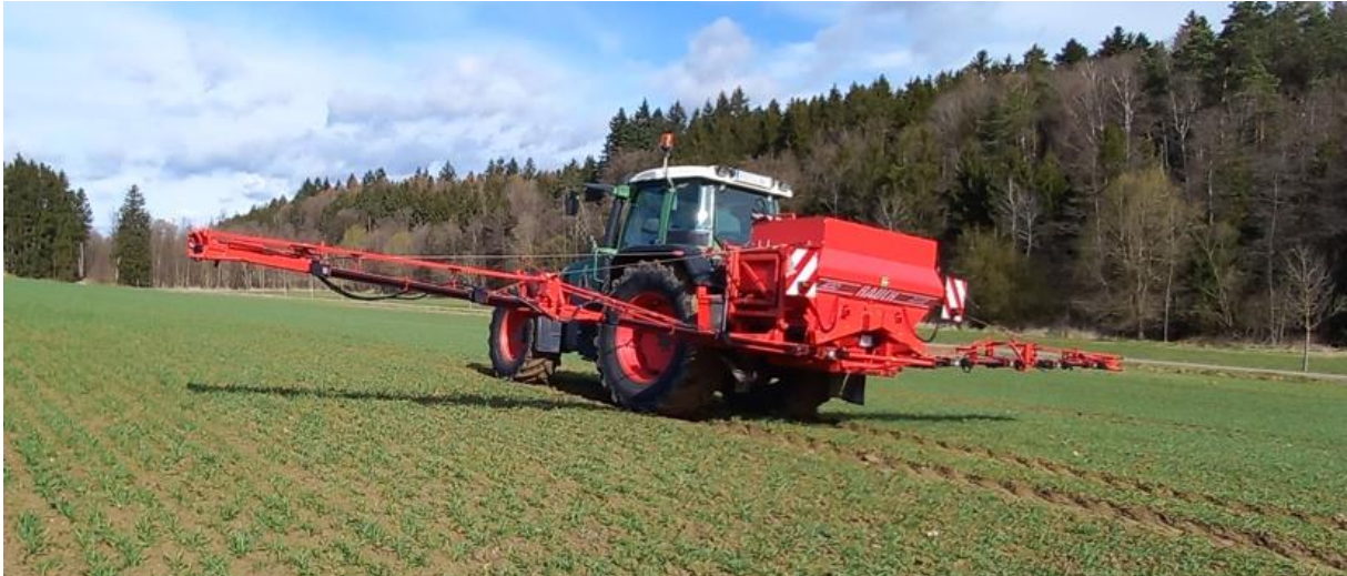
Figure 6: N-fertilizer application with the Rauch® AERO pneumatic spreader in winter wheat.
