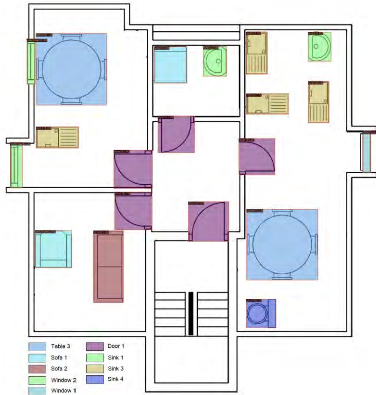
Figure 5.6: Sample from SESYD dataset with ground truth and highlighted furniture class objects MISHRA et al., 2021
