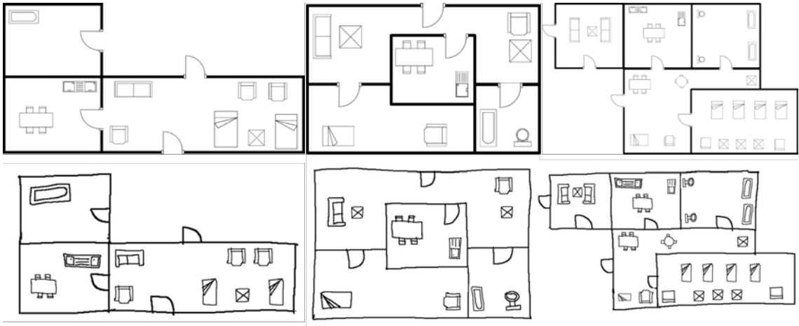
Figure 5.4: Samples from each category of the ROBIN dataset with the floor plan image on top and the matching sketch below D. SHARMA et al., 2017
