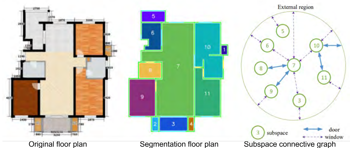
Figure 3.5: Vectorization steps based on EdgeGAN including the original floor plan, its segmented version and the subspace connective graph DONG et al., 2021
