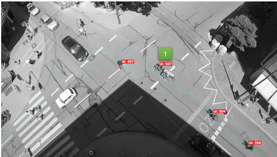
Figure 2.5: Study intersection Oberanger / Rosental / Rindermarkt (Munich, Germany) Bicyclist left arm hand gesture (explicit communication) combined with a stop inside the intersection area for a conditionally compatible left turn maneuver (1).
