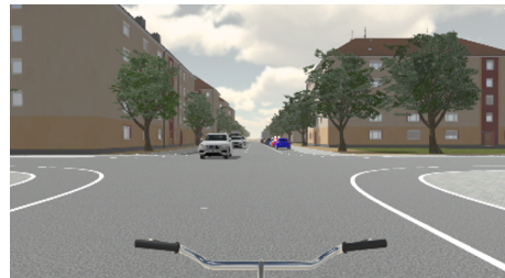
(d) The Bicycle Simulator by ANDREAS KELER, J. KATHS, et al. [2018] 3D Environment using DYNA4 coupled with SUMO
