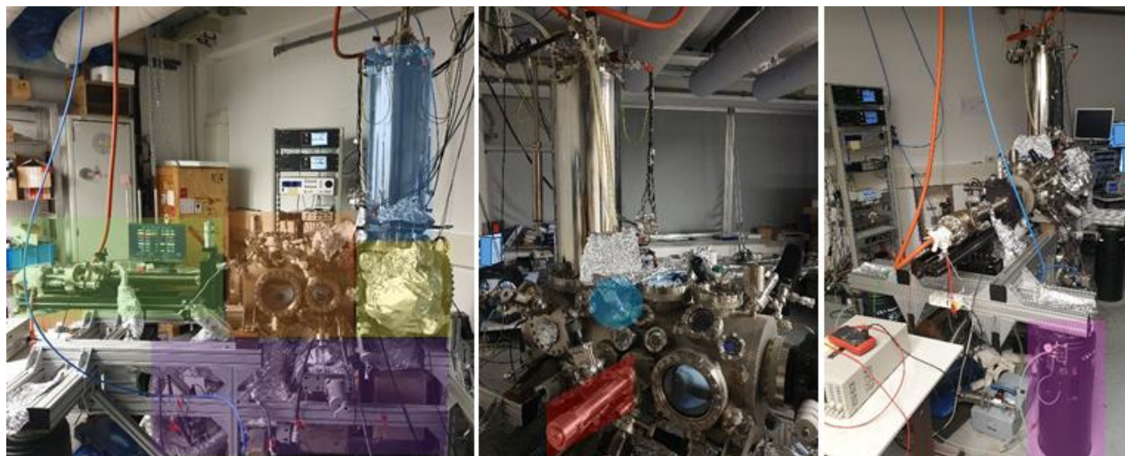
Figure 2.4 STM/AFM microscope. In the left image, indicated by different colors are the next sections: green-manipulator, orange-preparation chamber, purple-vacuum pumps, yellow-SPM chamber, blue-cryostat. In the middle image, indicated in red is the outer magnet that moves the sample parking lot, in blue the outer section of a custom made shutter. In the right image indicated in violet is one of the 4 pneumatic dampers.
