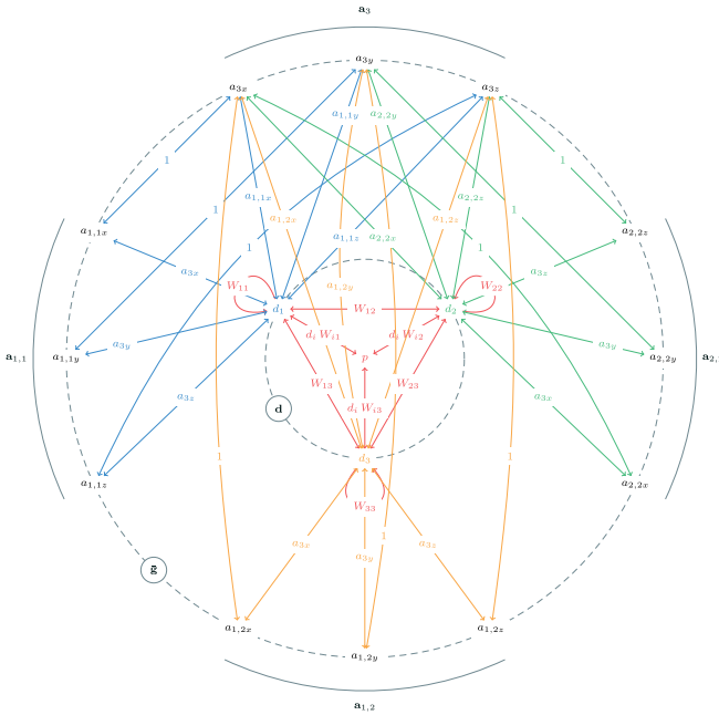
Figure 5.17: Computational graph of a shell element. Suboperations: p (red), d_1 = a_{11} - A_{11} (blue), d_2 = a_{22} - A_{22} (green), d_3 = a_{12} - A_{12} (orange).
