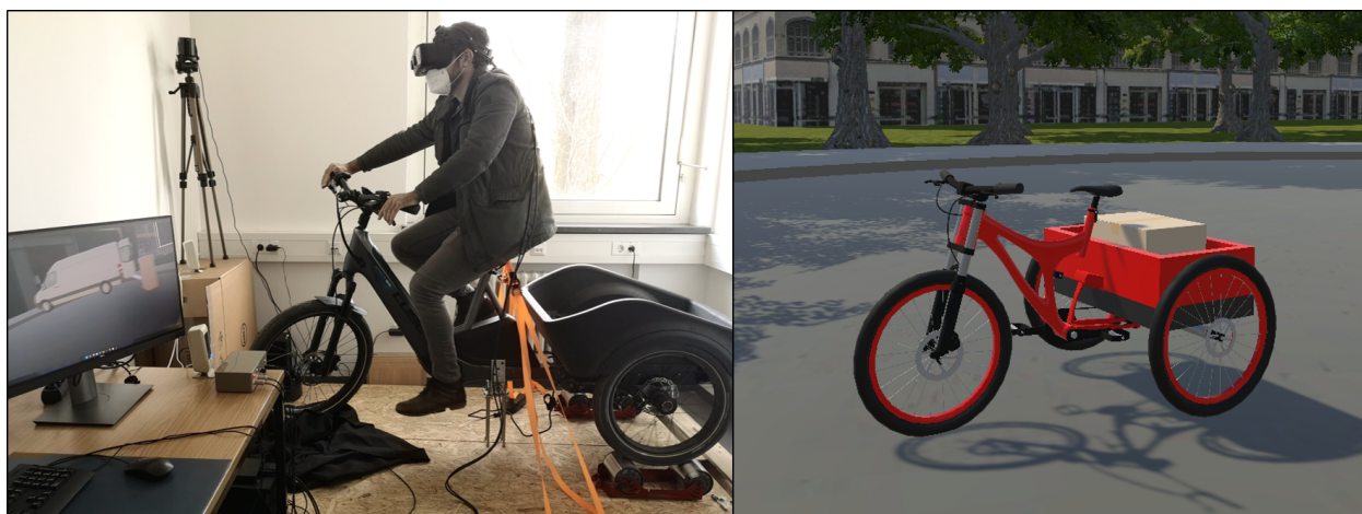
Figure 1: Cargo bicycle simulator (left: simulator setup, right: virtual model in Unity 3D)
