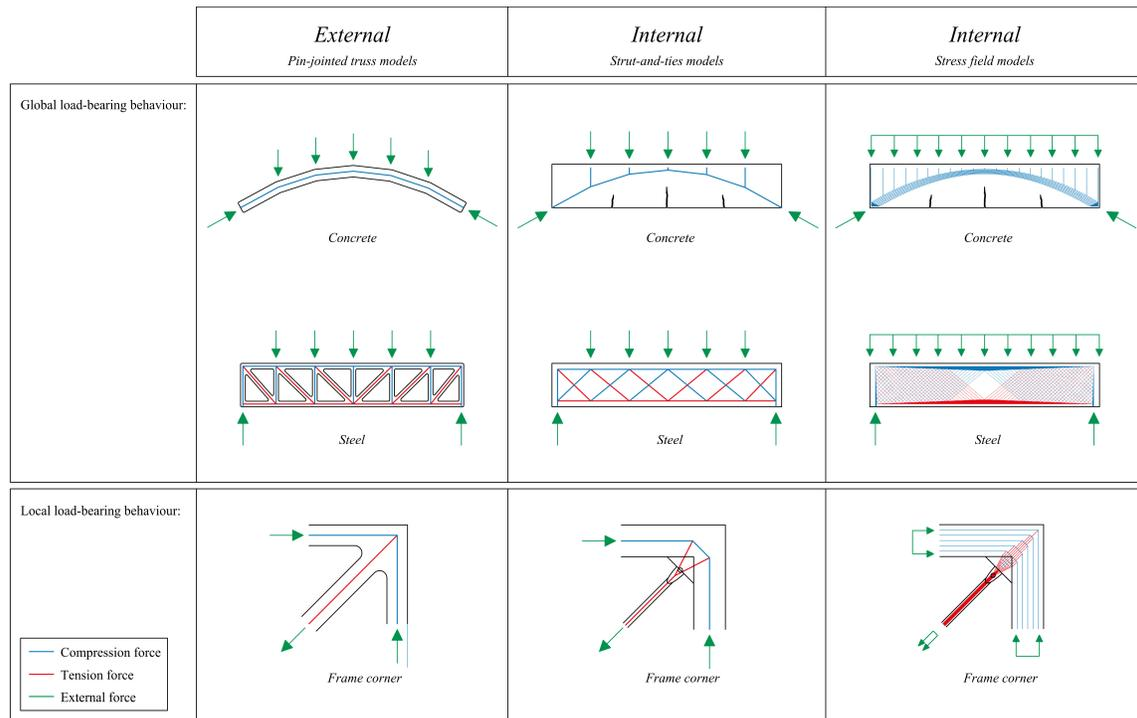
Figure 2: Equilibrium-based design allows dealing with different structural typology, materials or scales by respecting the three basic conditions of the lower bound theorem of plasticity theory.
