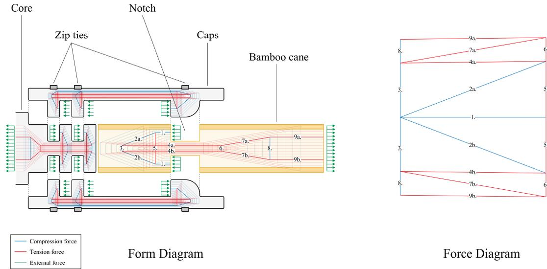
Figure 10: Illustration of the force flow in a connection under tension in the form of strut-and-ties and stress fields. Once the critical forces causing the failure in the bamboo have been identified (here 2. and 5.), it is possible to optimize the connection by adjusting its geometry, thus reducing the magnitude of the critical forces.
