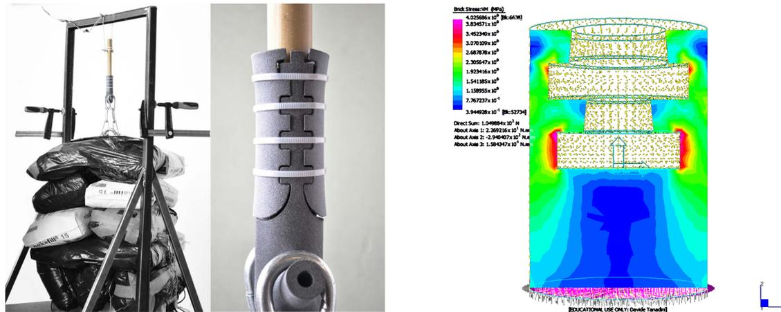
Figure 12: To validate the equilibrium-based design and analysis of the connection system, mechanical tests (left) and FE simulations (right) were performed. In the mechanical tests, cement bags (20 kg) are added incrementally. For the FE simulations, the software Strand7 [13] was used.
