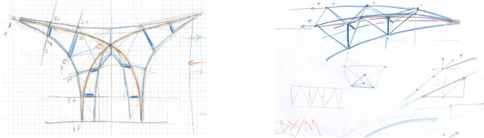
Figure 5: A sketch of the global structural system of the Digital Bamboo pavilion (left) and a conceptual study of the effect of post-tensioning on the space frame (right); red-tension, blue-compression.
