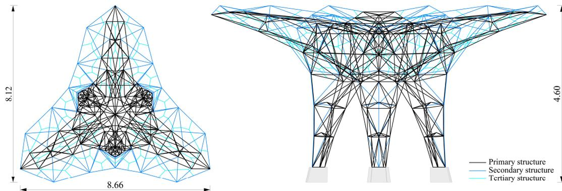
Figure 4: The hierarchical space frame structure of Digital Bamboo is composed of primary, secondary and tertiary sub-structures.
