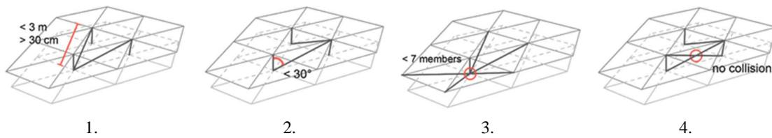
Figure 7: Overview of the rules adopted in the design of the space frame of the Digital Bamboo. Rules 1 and 2 constitute metric constraints, while 3 and 4 represent topological constraints.
