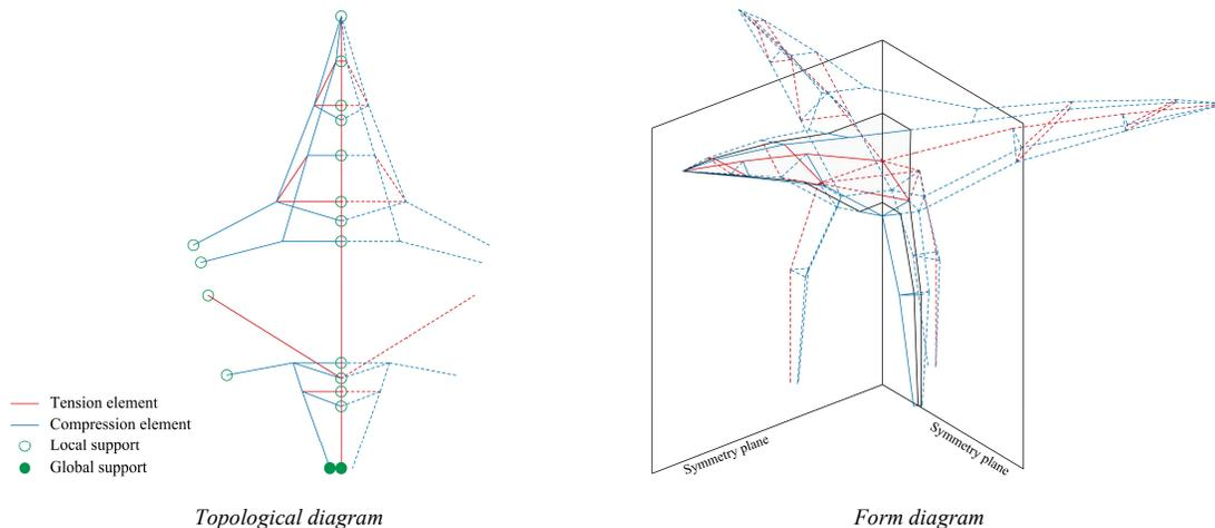
Figure 6: Only one-sixth of the primary sub-structure (continuous line) was generated using the Combinatorial Equilibrium Modelling (CEM) [11] and then mirrored using symmetry planes.
