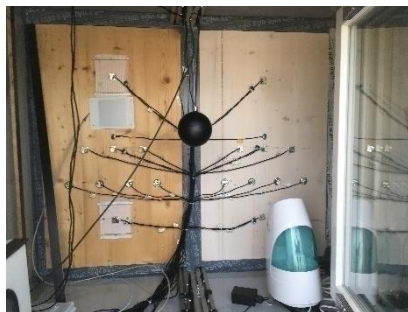
Figure 1: Measurement setup for the experiments in the test cube with two facade test elements: untreated (left) and glazed cross-laminated timber surface (right). The humidifier shown was not used for the analyzed period.
