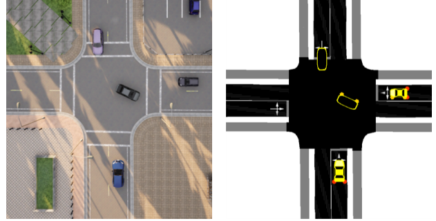
Fig. 3. A scenario in the CARLA simulator (left) and SUMO simulator (right). The states of the ego vehicle (blue car) and other road users are synchronized between CARLA and SUMO.
