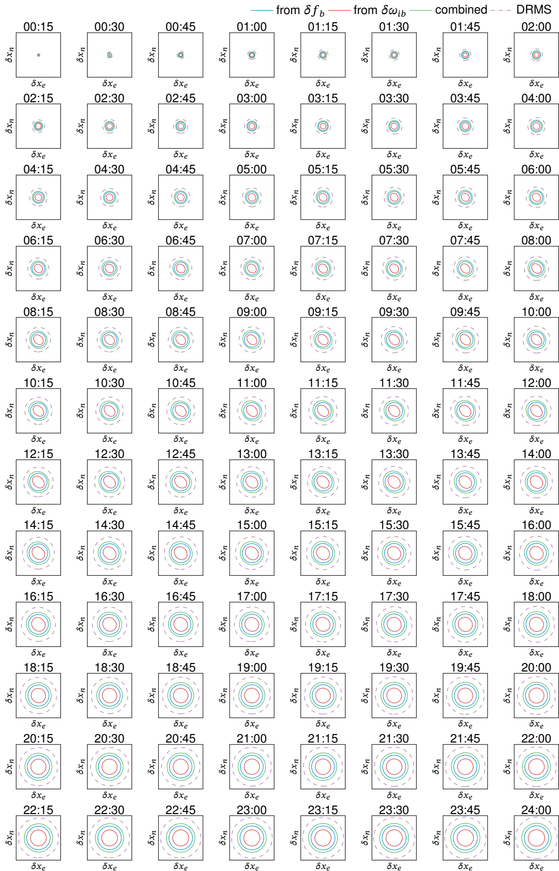
Figure 3.26.: Development of the horizontal position covariance from isotropic 1 \text{ mg}/\sqrt{\text{Hz}} accelerometer and 0.0017^\circ/\sqrt{\text{h}} gyroscope random walk at \phi = 45^\circ and \psi = 0^\circ .
