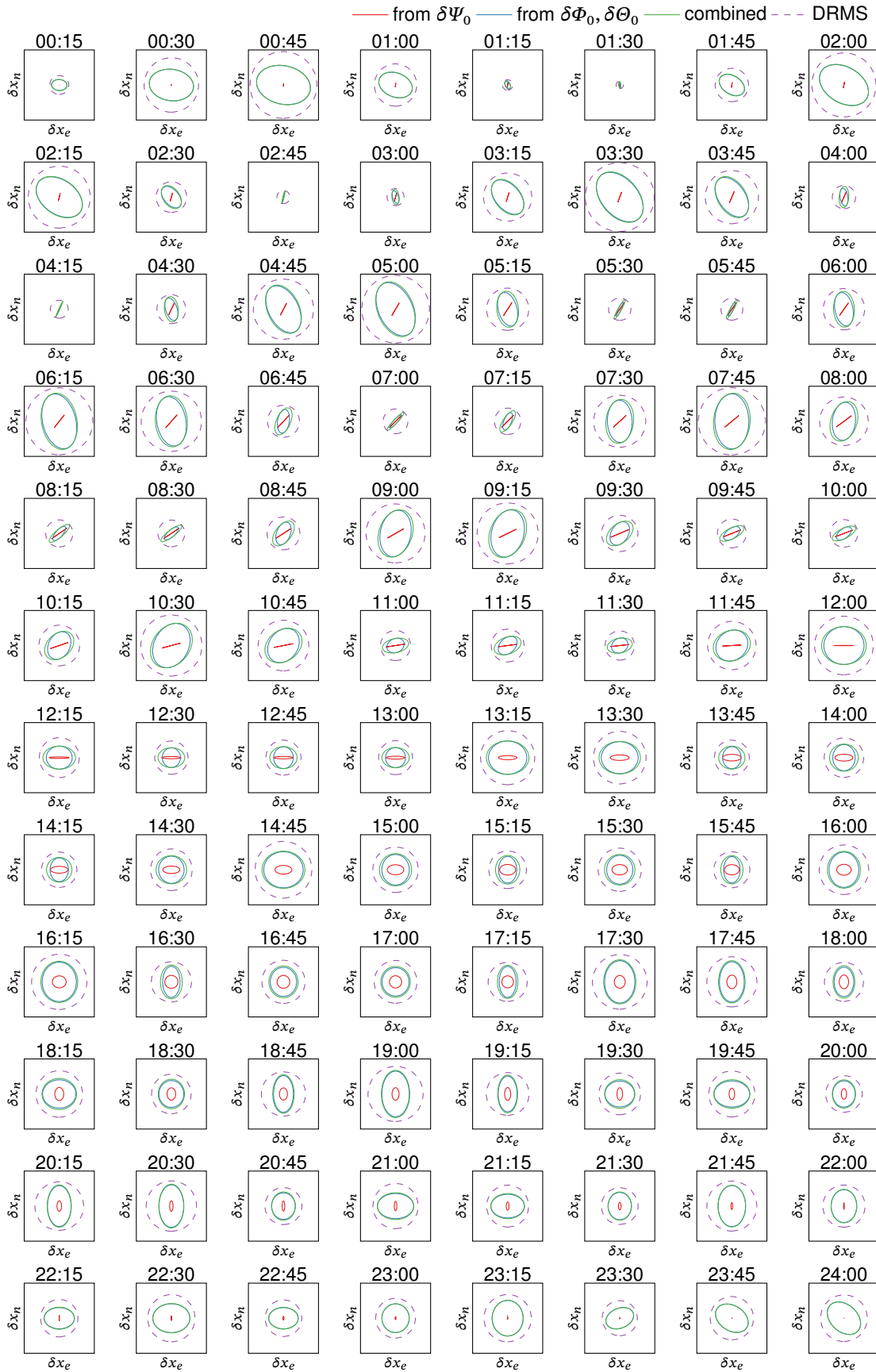
Figure 3.11.: Development of the horizontal position covariance from correlated 0.01^\circ initial pitch and roll ( 1\sigma ) and 0.01^\circ ( 1\sigma ) yaw alignment error at \phi = 45^\circ and \psi = 0^\circ .
