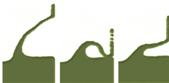
Figure 2.1.: Three liquid surfaces after 60 time steps differing only by \pm\epsilon in initial conditions. Even this initially minimal difference can lead to large differences in surface position.
