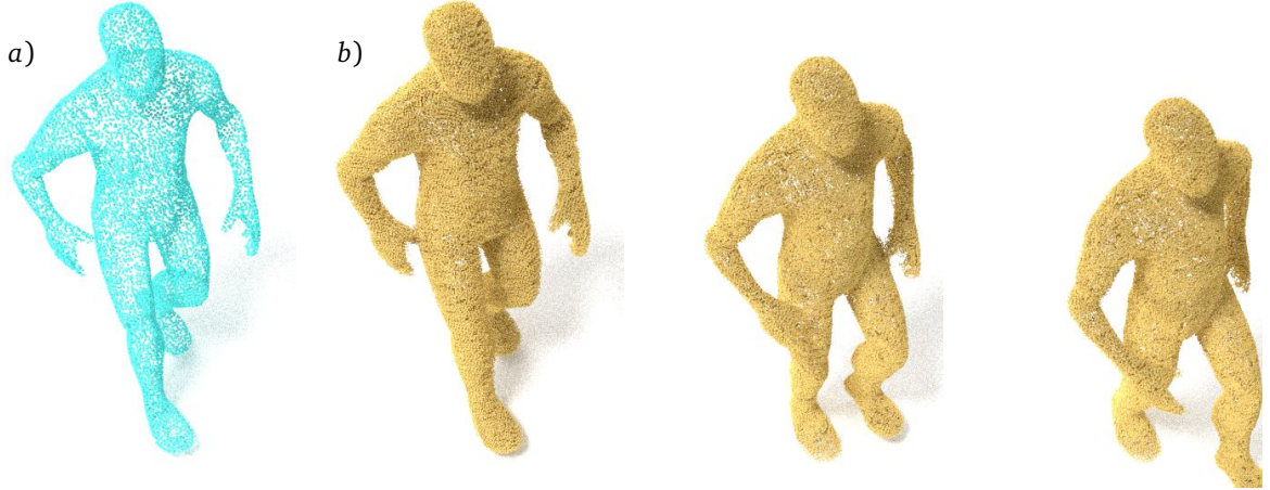
Figure 3.7.: Our algorithm upsamples an input point cloud (a) in a temporally coherent manner. Three exemplary outputs in (b).
