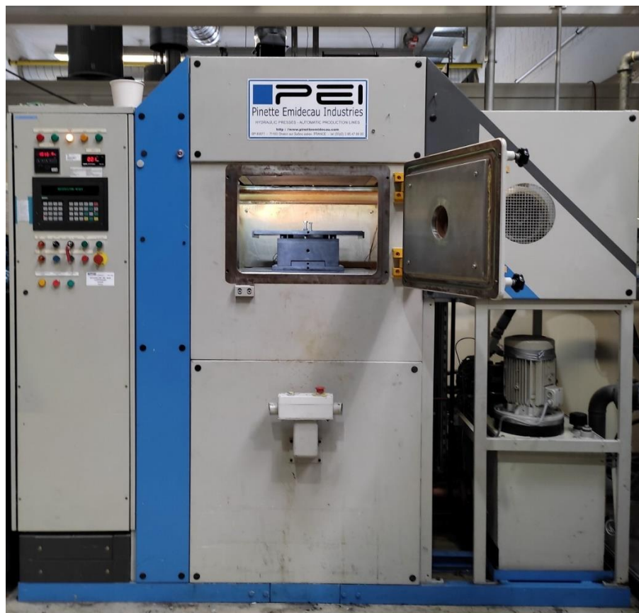
Figure 3-4 The 100-ton laboratory press with mould placed inside
