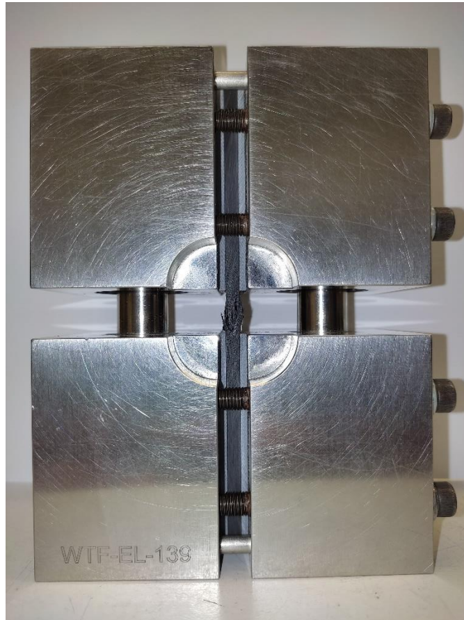
Figure 4-14 Combined loading compression fixture with a sample installed, after testing, strain gauge wires already removed
