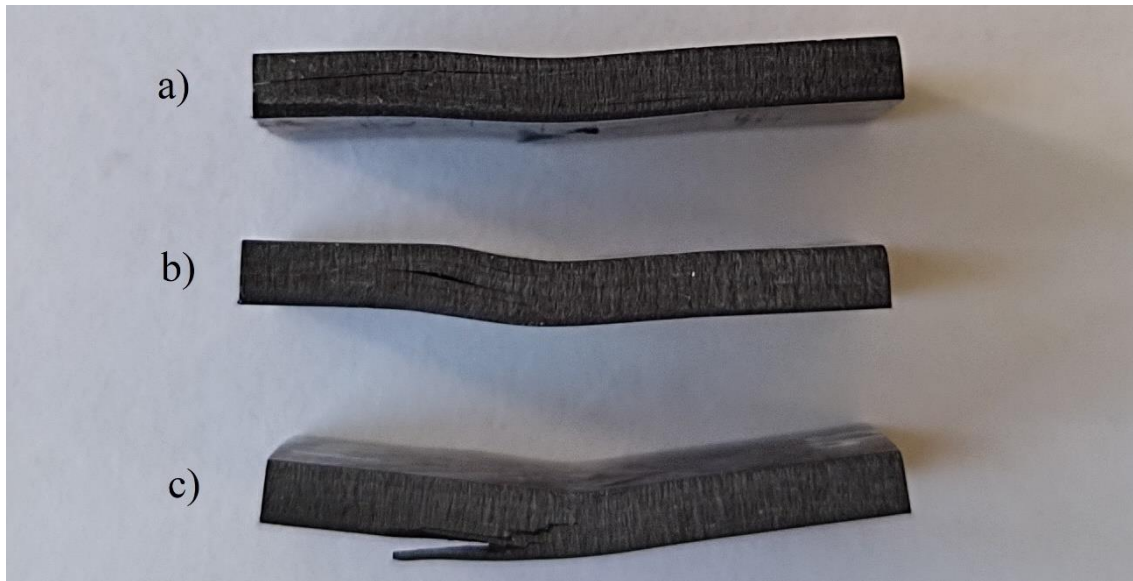
Figure 4-19 Failure modes of ISO 14130 samples: a) partial interlaminar crack from left side towards middle, tensile break; b) plastic deformation and partial layer separation; c) pure tensile break of the bottom most layer
