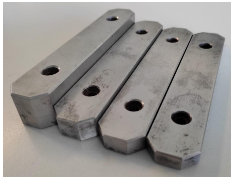
Figure 3-7 Distance blocks for 20mm, 10mm, 6mm and 4mm thick plates
