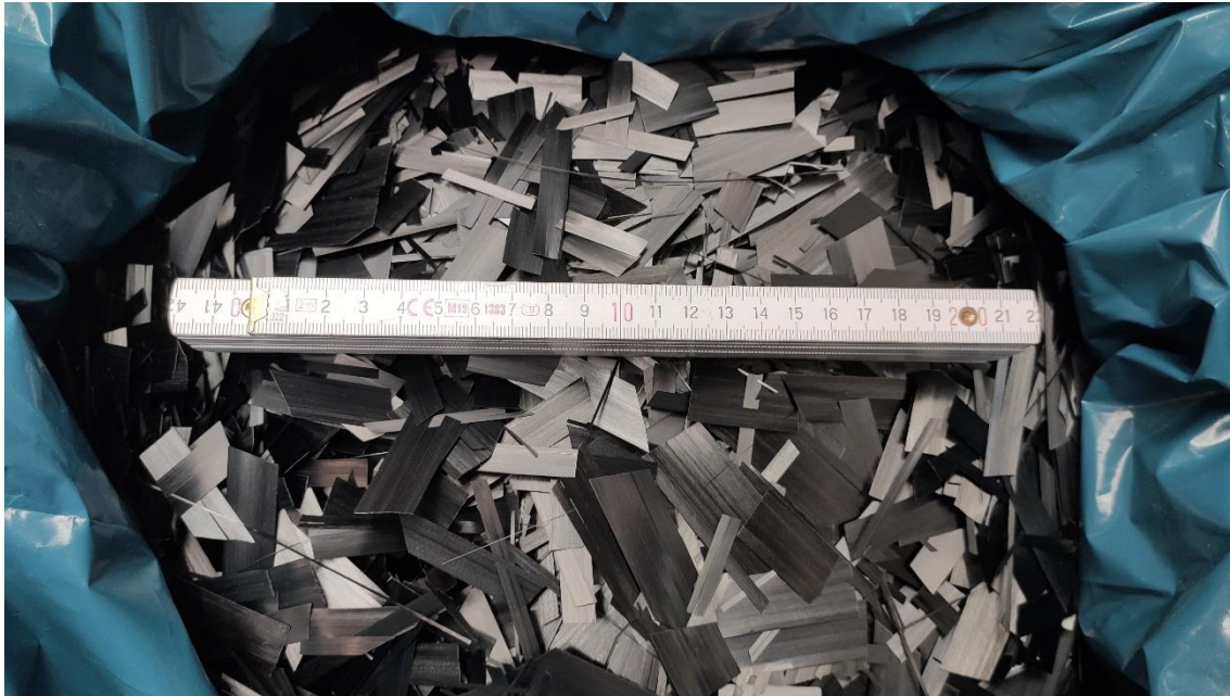
Figure 3-1 CF-PEEK tape scraps that serve as basis for the recycling process
