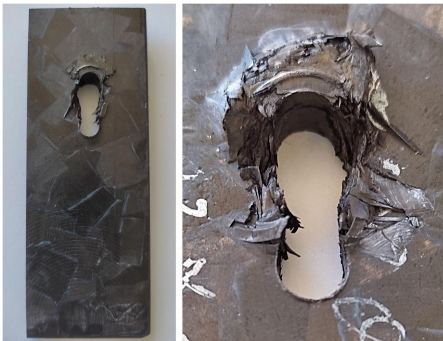
Figure 4-22 Plain pin bearing strength sample P4809 tested beyond its yield point: Left – complete sample; Right – close up of tested area
