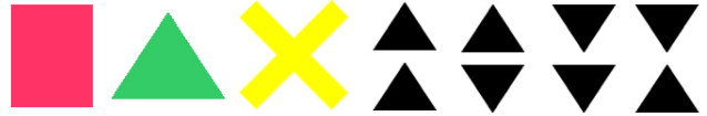
Fig. 3. Visualization of supported traffic signs. From left to right: two lateral marks, special mark, and cardinal marks for north, east, south, and west.
