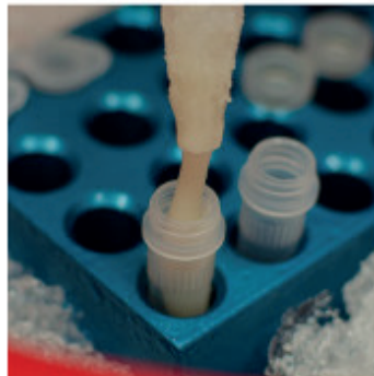
Figure 1.3: A bacterial cell suspension containing glass beads is filled in a 2 ml bead beating tube. The suspension shows high viscosity. The figure was adapted with permission from [59].
