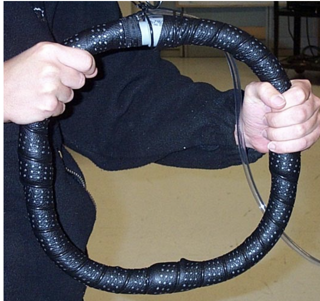
Figure 2.9: Haptic steering wheel [used by Enriquez et al. (2001)]. Built from PVC conduit and a vinyl steering wheel cover; the pneumatic display is located beneath the steering wheel cover, under the subject's right hand. (Fig. and caption taken from Enriquez et al. (2001))
