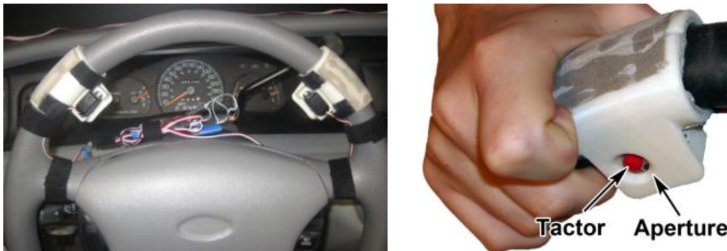
Figure 2.11: (left) Tactile feedback devices as haptic input mounted to the driving simulator's steering wheel. The shear tactors face towards the dashboard. (right) User's hand gripping the steering wheel. The index finger is retracted to more clearly show the tactile interface. (Fig. and caption taken from Medeiros-Ward et al. (2010))
