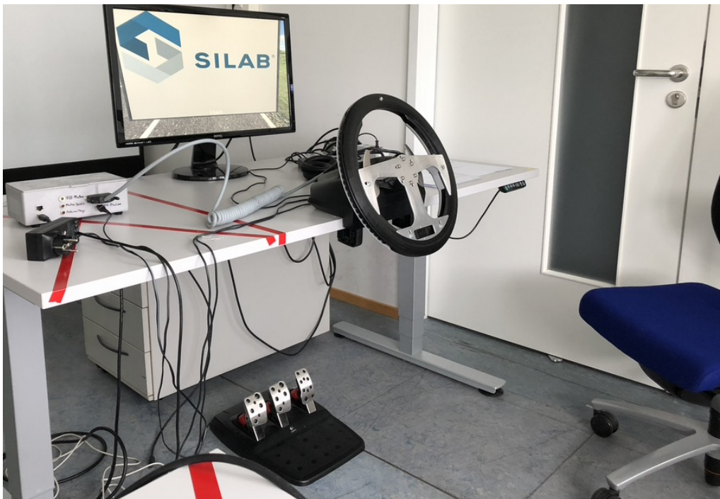
Figure 4.2: Participants table with the display, TWG on the Logitech G27 base, pedals under the table and chair on the right.
