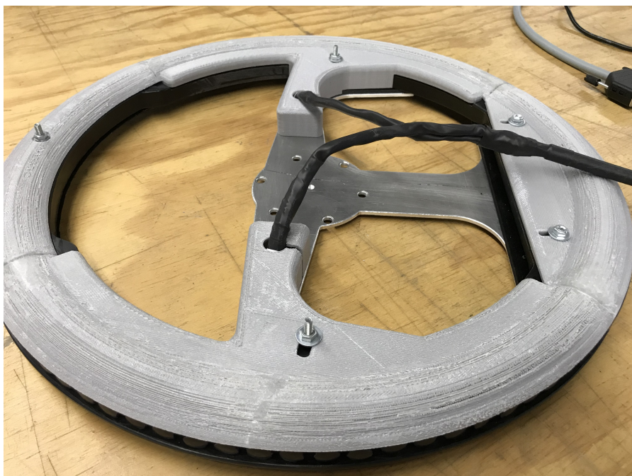
Figure 3.17: Back view of the final prototype with the taped together solenoid cables in black. (Fig. taken from Broers (2019))
