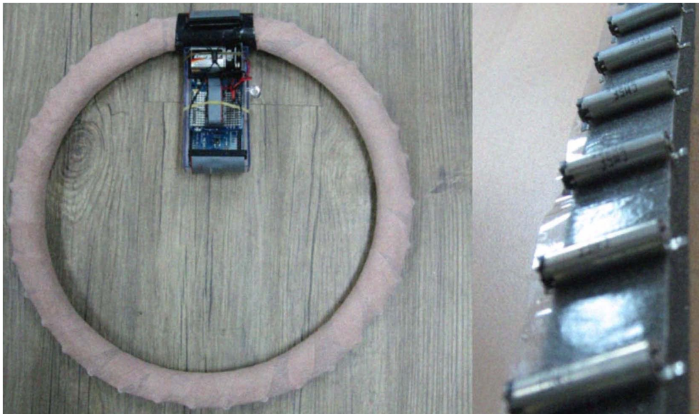
Figure 2.6: 32 vibration motors spread out across the steering wheel used by Hwang and Ryu (2010) (Fig. taken from Hwang and Ryu (2010))
