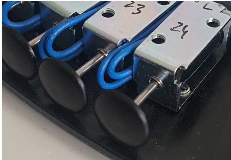
Figure 3.9: Close up view of the plastic caps installed on the solenoids pins. (Image taken by Christofer Keppler)
