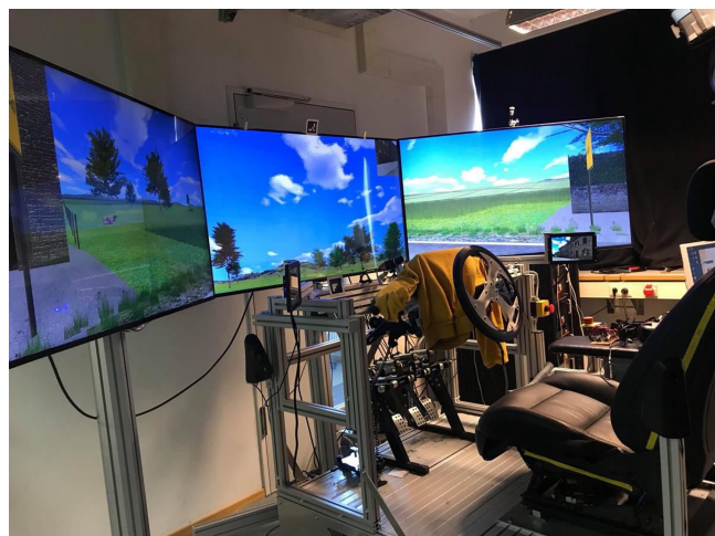
Figure 3.13: Setup of the second evaluation: TWG mounted in a seat bucket. (Fig. taken from Bahri (2019))
