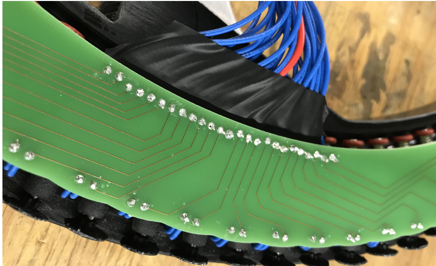
Figure 3.16: Custom made circuit board mounted on top of the solenoids. (Fig. taken from Broers (2019))
