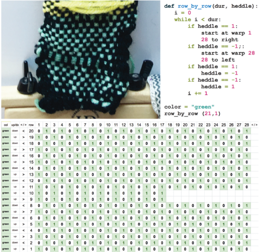
Figure 3. Devanie’s plain weave (top left), the analytical pseudocode translation by the researcher (top right), and the bitmap translation (bottom) of Devanie’s project.
