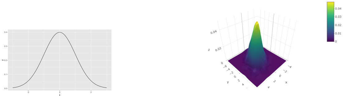
Figure 1: The left graph is univariate Gaussian density for a variable X \sim \mathcal{N}(0, 1) and the right one is multivariate Gaussian density over two variables (X, Y) \sim \mathcal{N}_2(\mathbf{0}, \Sigma) , where \Sigma = (3, 2; 2, 5) .
