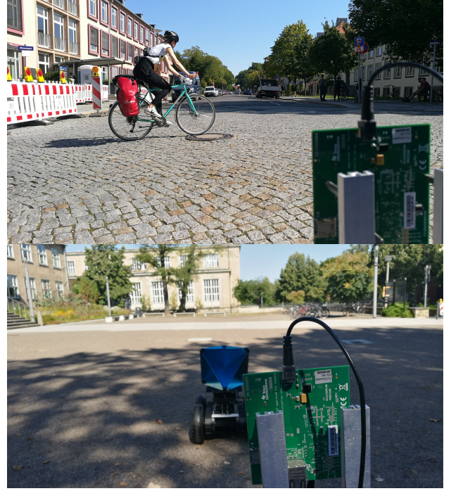
Fig. 4: Images with the two setups used for experimental radar recordings. On the top image, the radar faces objects with different radar cross-section. On the bottom image, the radar faces a mobile robot carrying a corner detector.
