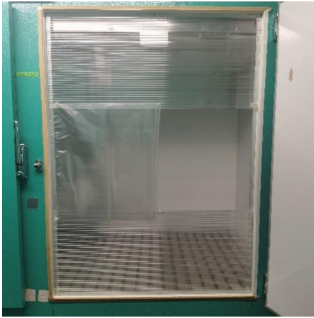
Fig. 2.2 Picture of air-lock. One air-lock consists of two PVC plates (770 × 460 mm) and two plastic sheets (570 × 400 mm). Two PVC plates were installed above and below the door. The middle area was left for the operation window, covered with two plastic sheets. The air-lock covered the growth chamber door completely.
