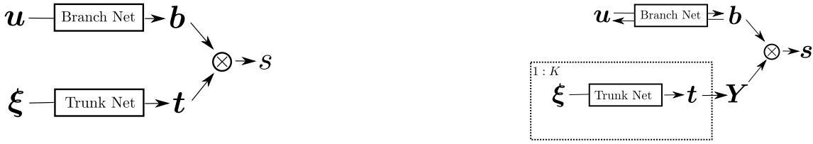
Fig. 1 (Left) Classical DeepONet (Lu et al, 2019) and (Right) proposed Invertible DeepONet architecture
