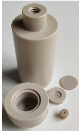
Figure 55: Rotor packing tool adapted for compatibility with the Bruker rotor grabber, disassembled.
