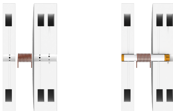
Figure 8: Illustration of the rotor-stator system used in MAS NMR probes. Left: Stator and coil without an inserted rotor. The parts of the stator immediately next to the coil form the air bearing, while the rightmost part contains the drive system that acts on the turbine fins of the rotor top cap. Right: Stator with inserted rotor.
