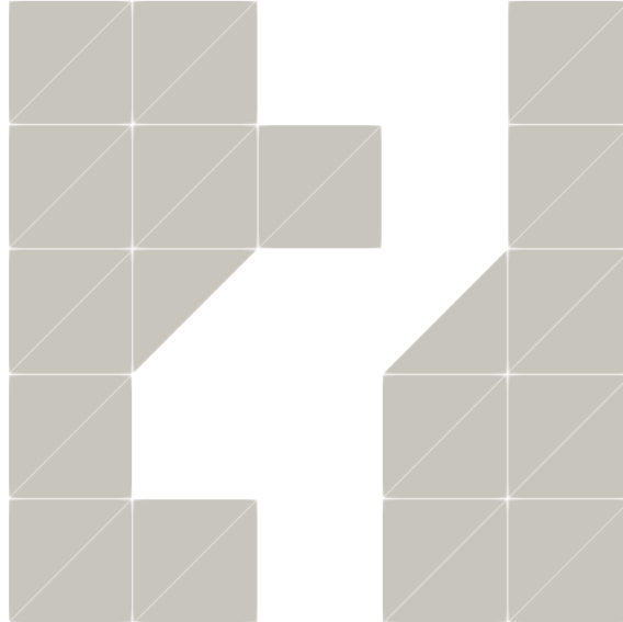
Figure 2.5.: Example of missing connectivity: a triangulation of the unit square with 2 ranks. When no rank owns the 3 vertices of a triangle, this triangle is discarded. This occurs if no duplication is implemented.
