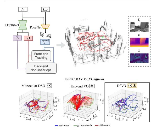
Figure 8.1: We propose D3VO – a novel monocular visual odometry (VO) framework which exploits deep neural networks on three levels: **D**eep depth (D), **D**eep pose  $(T_t^{t-1})$  and **D**eep uncertainty  $(\Sigma)$  estimation. D3VO integrates the three estimations tightly into both the front-end tracking and the back-end non-linear optimization of a sparse direct odometry framework [15].
