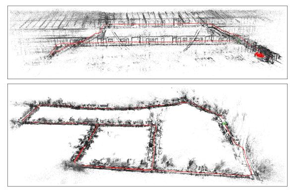
Figure 2.1: Trajectories and pointclouds estimated by DM-VIO. Top: Magistrale of our office building reconstructed using a sequence from the TUM-VI dataset. Bottom: A sequence from the automotive 4Seasons dataset. Long stretches of constant velocity constitute a challenge for monocular visual-inertial odometry, but thanks to our novel IMU initializer, the method works very well.
