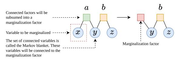
Figure 3.2: Factor graphs before and after marginalization of variable x. The marginalization factor replaces all connected factors and is connected to the variables which form the Markov blanket of x.
