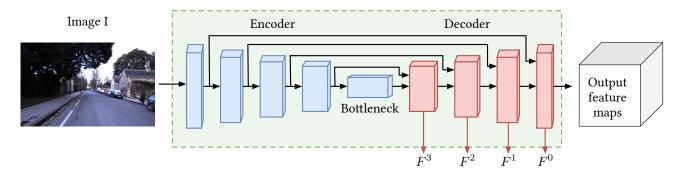
Figure 6. Overview of one branch of the Siamese network architecture. Each branch is a modified U-Net [5] architecture which receives as an input an image and predicts multi-scale feature maps  $[F^0, F^1, F^2, F^3]$ . The multi-scale feature maps from the decoder network of both branches are then passed and used by DSO. Note that the weights between the two branches are shared.
