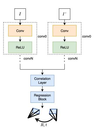
Figure 1: Network architecture of CorrPoseNet.
