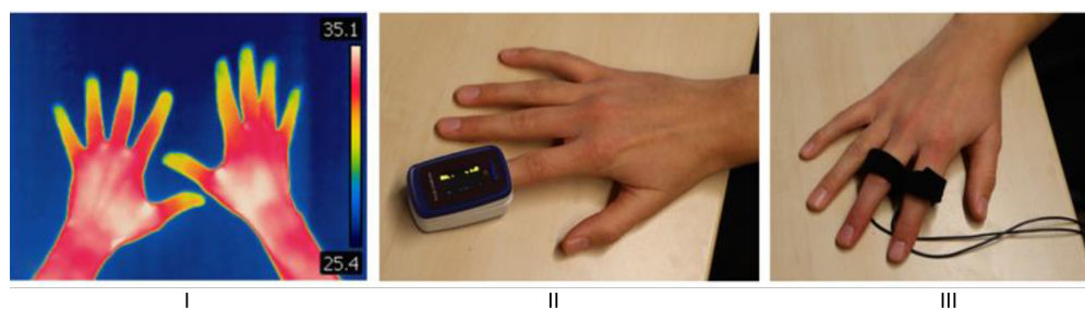
Figure 4. Used measurement tools for additional patient monitoring. Displayed are (I) the temperature by Seek Thermal CompactPRO, (II) pulse oximeter (PULOX PO-200), and (III) skin conductance.
