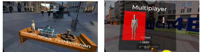
Figure 7: (Left side) VR travel App based on interactions with 3D objects, which need to be touched by the walking stick to travel to other places; (right side) Multiplayer setup with 3D avatars based on images taken of the person
