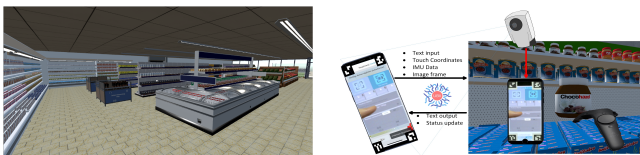
Figure 6: VR supermarket: (left side) shows the authentic virtual environment with realistic German products and store layout; (right side) Augmented Virtuality setup used with mobile health apps on the physical smartphone
