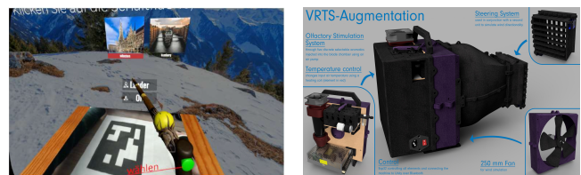
Figure 8: (Left side) Augmented Virtuality in use to prevent disorientation and panic reactions and the selection method based on a walking stick; (right side) System to generate warm or cold airflow with changing directions and through the use of essential oil bottles different types of odours are created
