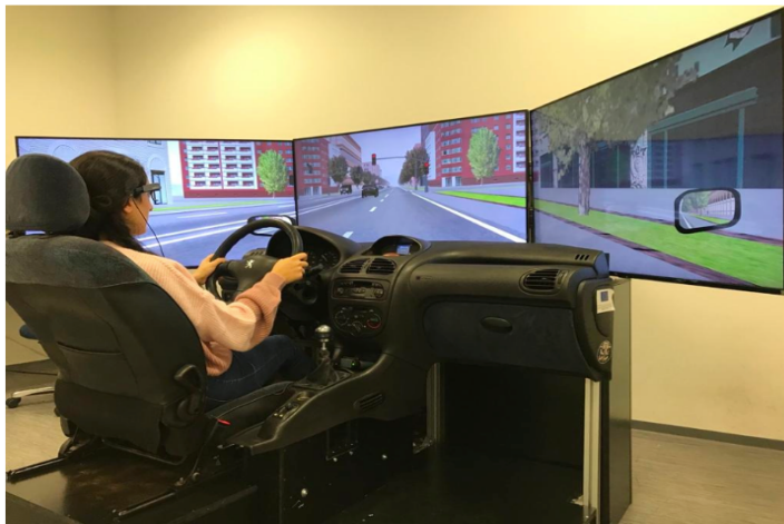
Figure 10 i-DREAMS driving simulator, Chair of Transportation System Engineering (TSE, 2021)
