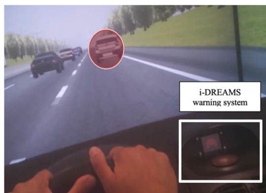
Figure 11 i-Dreams warning system and eye movement (red dot)
