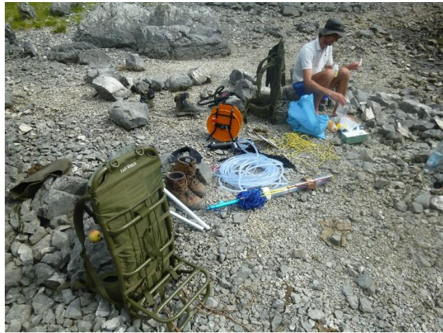
Figure 9: The picture shows some central equipment of the lake sampling: Gravity corer, hose sampler and hydrophysical multiprobe as well as carriage systems. In the background, water samples are pre-processed on site using syringe filters. Photo credit: Lorenz Tschampel.
