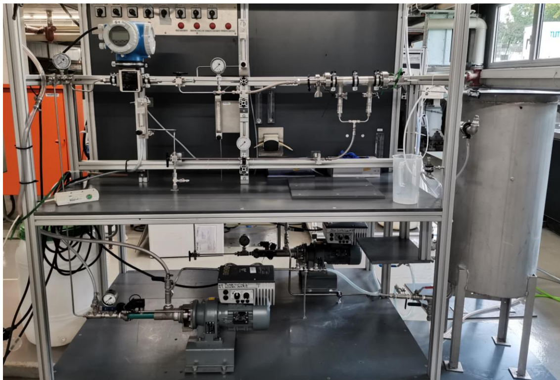
Figure 11-8: Photo of lab-scale UF membrane system
