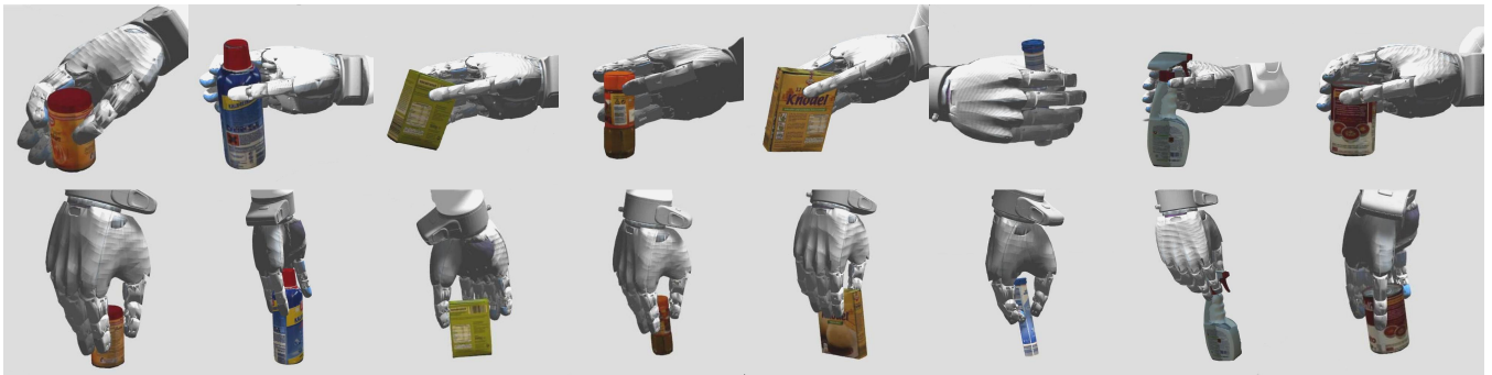
Fig. 6: The successful grasp poses generated from FFHNet for eight test objects in simulation. Each column represents one unknown test object. For each object, our FFHNet model is able to predict both top (first row) and side grasps (bottom row).
