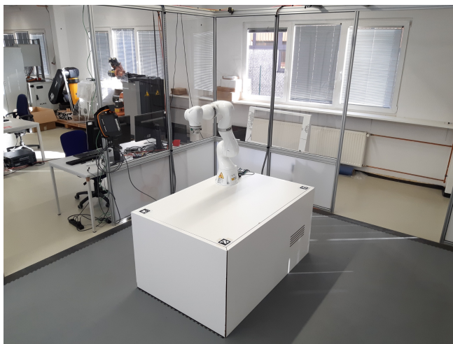
FIGURE 4: Kuka LBR iiwa collaborative robot mounted on a worktable inside our workcell dedicated for research purposes. We use multiple Kinect v2 depth sensors mounted in the corners of the workcell to get full coverage. The extrinsic calibration, i.e. point cloud registration, of the 3D vision system is performed with our proposed method, because it provides robust and accurate alignment due to the object-centric approach. Additionally, for the indoor real-world scenario, we assume that the movement of the object of interest, in our case the robot arm, cannot cause any significant positional discrepancy in the depth sensors. This assumption is valid because the time synchronization of multiple connected depth sensors is usually by magnitudes faster than the movement of any object within a scene.
