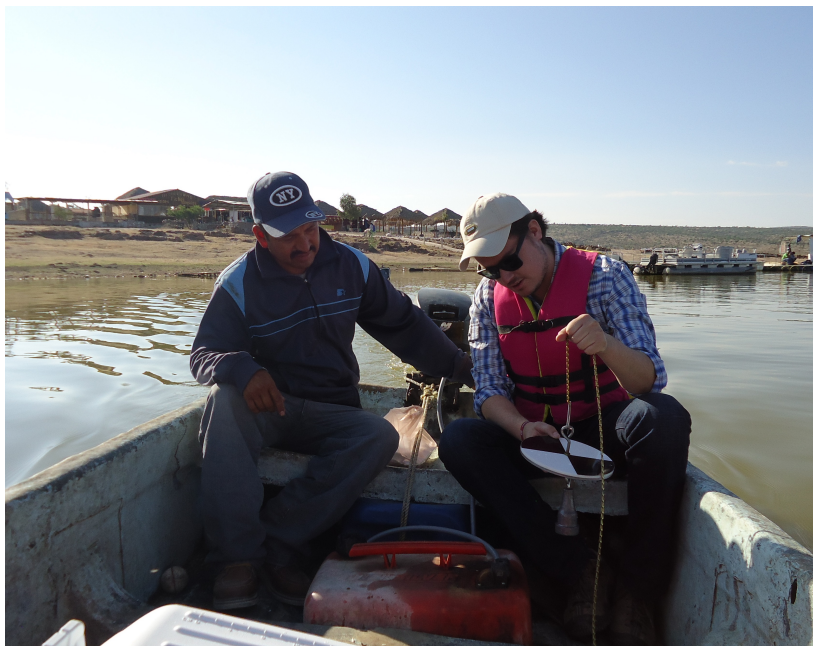
Figure 2.5: Conventional measurement of transparency by the author using a Secchi Disk (2013). Location: Plutarco Elias Calles Reservoir, Aguascalientes, Mexico ( https://goo.gl/maps/sjjbgq9aZGUVjNZn9 ).
