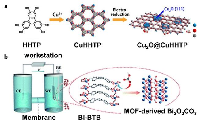
**Figure 9.** Schematic illustration of the *In-situ* electrochemical transformation of pristine MOF to obtain MOF derivatives: a) partially conversion; Copyright 2020, Wiley-VCH Verlag GmbH & KGaA, Weinheim; Reproduced with permission from Ref. [89]. b) fully conversion. Copyright 2021, Royal Society of Chemistry. Reproduced with permission from Ref. [90].
