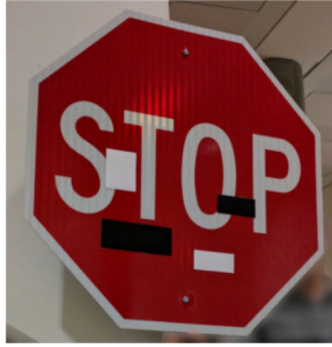
Figure 2.4: An adversarially perturbed stop sign by Evtimov et al. [32], which is classified as 'Speed Limit 45mph'.
