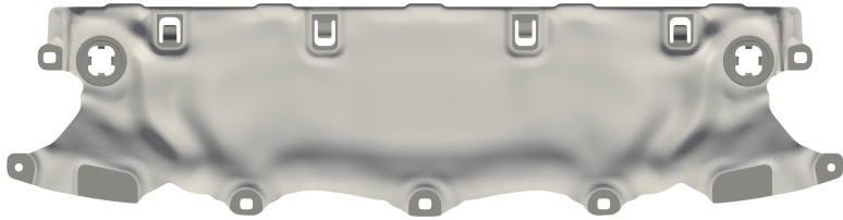
(a) Optimal design after shape optimization of leveled design.
