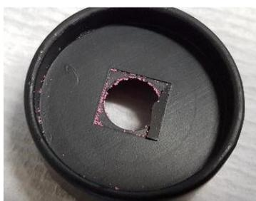
Figure 16. Pink polystyrene particles accumulated at the rim of and adhered to a silicon filter adapter. A piece of a broken membrane at the right. Photo: Lerch (2020).
