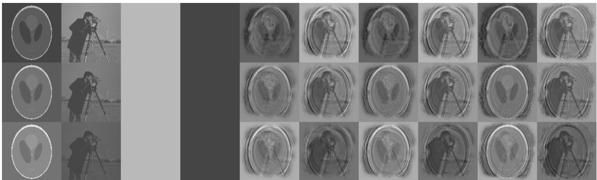
Figure 6.21: Reconstruction of the object for blind polychromatic ptychography. Each row corresponds to a single frequency \ell = 0, 1, 2 . The two consecutive columns are the real and imaginary parts of the object. In the figure, we show the true object x and iterates z^t of Algorithm 13 for t = 0, 10, 50, 200 .
