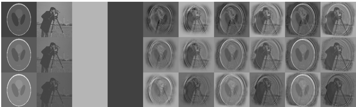
Figure 6.18: Reconstruction of the object with a known window. Each row corresponds to a single frequency \ell = 0, 1, 2 . The two consecutive columns are the real and imaginary parts of the object. In the figure, we show the true object x and iterates z^t for t = 0, 100, 500, 2000 .
