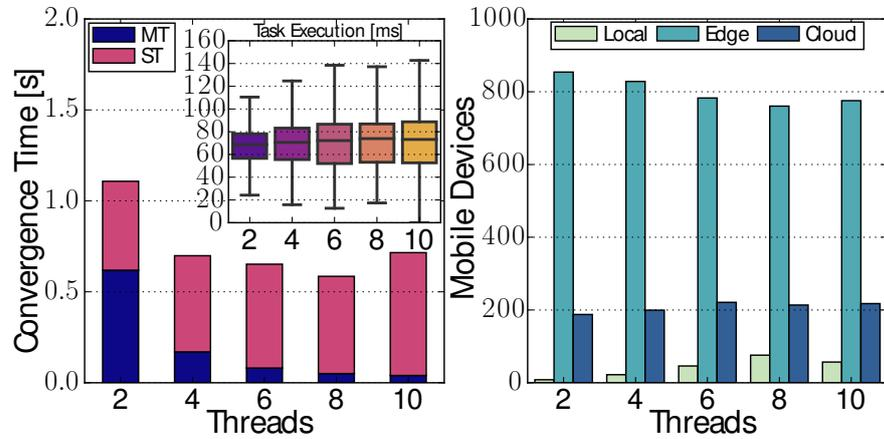
Figure 4.30: Performance of 2PMT-Nimbus (Multi-threaded (MT), Single-threaded (ST)).
