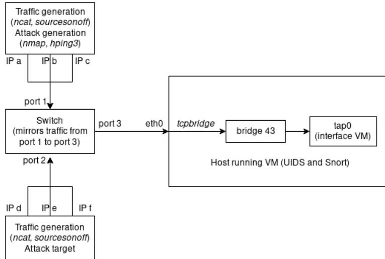
Figure 3.4: Setup for live traffic.
