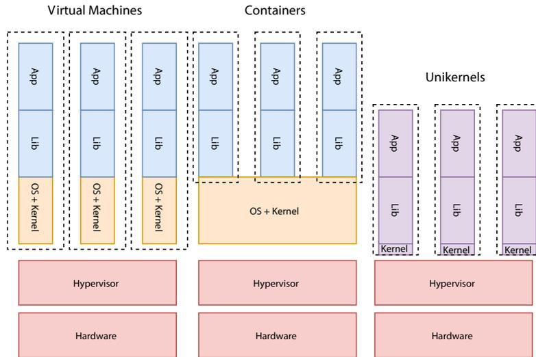
**Figure 4.2:** Comparison of different virtualization technologies.
