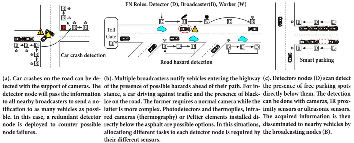
Figure 4.12: ECCO example use-cases. (a) Car crash detection, (b) road hazards detection, (c) smart parking.
