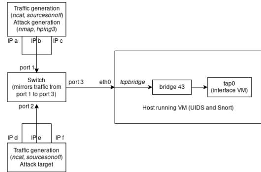
Fig. 3. Setup for live traffic.
