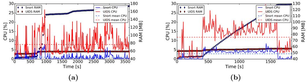
Figure 3.6: UIDS vs. Snort (CICIDS2017, RPI) — Port scans (a) and DoS (b).
