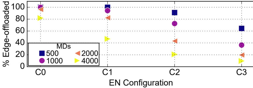
Figure 4.28: Fraction of task offloaded to the edge.
