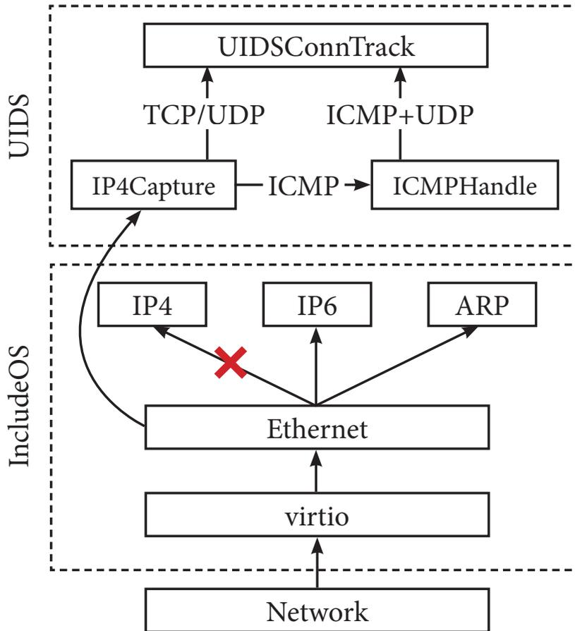
**Figure 3.2:** UIDS structure and packet reception path.
