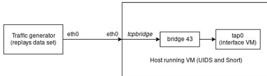
Fig. 2. Setup for traffic replay.
