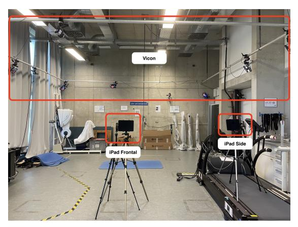
Figure 2.3: Camera setup of laboratory experiment B. The 14 Vicon infrared cameras are positioned around the subject close to the ceiling of the laboratory. Two iPads are positioned frontally facing the subject and in a 30° angle.
