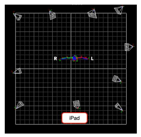
Figure 2.2: Camera setup of the laboratory experiment A. The subject is positioned at the center of the tracking area. 10 infrared cameras of the *Vicon* system are positioned around the subject. An iPad is positioned in front of the subject. "L" and "R" mark the subject's left and right body side, the subject is facing the iPad.
