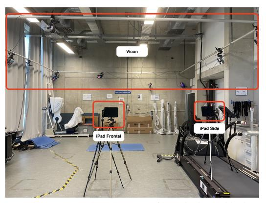
Figure 2. The experiment setup, showing the positioning of the recording devices and the subject.
