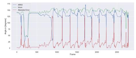
**Figure 11.** Left elbow angle of one of the subjects in the Single Leg Deadlift exercise, which shows several unexpected spikes during the execution. The spikes originate from ARKit incorrectly detecting the joint's position, most probably because of bad visibility of the elbow joint during the exercise.
