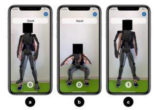
**Figure 4.** Exercise repetition tracking using the pose-based approach. ARKit's recognition is shown by the robot overlay. ARKit tracks the poses in a, b, and c, and updates the repetition count after pose c is matched.
