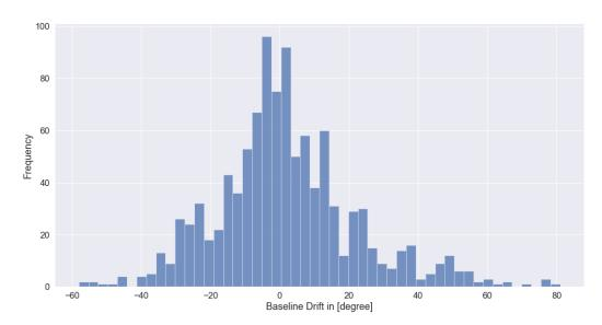
**Figure 9.** Results of the baseline drift analysis of the ARKit data. This is computed by minimizing the MAE by shifting the ARKit data vertically. The results show a normal distribution around 0, thus indicating no systematic baseline drift of the ARKit results.
