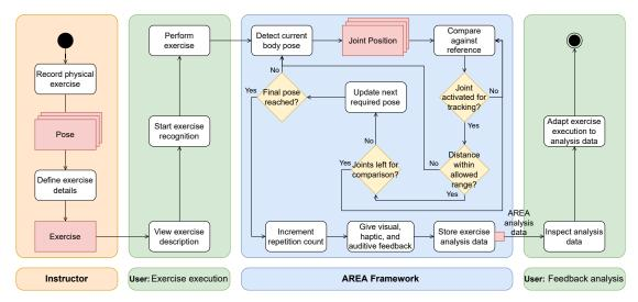
Figure 2.5: UML activity diagram representing the flow of events of the AREA algorithm. The diagram includes activities performed by the instructor to record a new exercise, the user by performing an exercise and analyzing their feedback, and the AREA framework recognizing and counting valid exercise repetitions.
