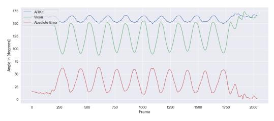
**Figure 7.** Left hip angle of one of the subjects in the Side Squat exercise in degrees. The plot shows that while the motion pattern is visible in both recordings, ARKit exposes a reduced amplitude and a shift on the *y*-axis.
