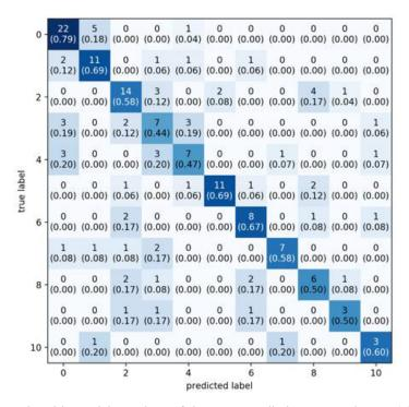
**Figure 3.** Confusion matrix with precision values of the CNN prediction on 11 classes: (0) Dive Right (1) Dive Left (2) Catch Hand (3) Catch Body (4) Catch Ground (5) Jump Catch (6) Jump Catch Run (7) Throw Low (8) Throw High (9) Side Kick (10) Side Kick Ground.
