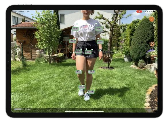
Figure 3.2: Woman being recorded by the *ARKit* system running on an iPad. The joints are detected by the camera and visualized on the screen including the detected joint angle in degrees.
