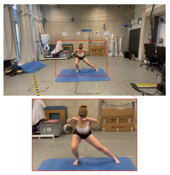
Figure 3.1: Woman being recorded by the *Vicon* system with reflective markers attached to her body. Infrared cameras are placed around the subject to capture the markers.
